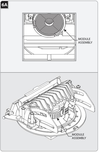
To adjust the height, grip the module assembly and push up to minimize glare and flash on the trim. Pull down on the module assembly for maximum light output and efficiency.
