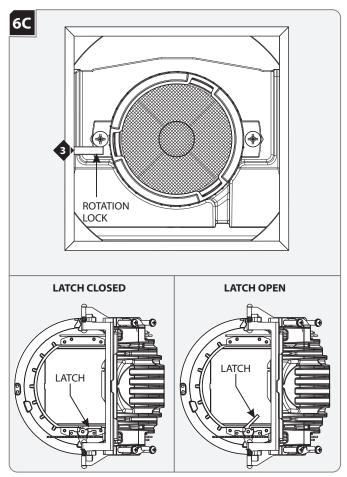
**NOTE:** Lamp housing can rotate 361° horizontally.
